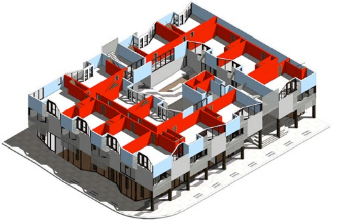
FIGURE 9: Example of Fire Rated walls using Data Visualization
